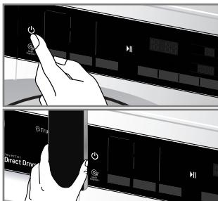
1. Press the Power button to turn on the washer. Do not press any other buttons or turn the cycle selector knob.
