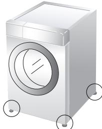
1. Leveling the washing machine properly prevents excessive noise and vibration. Install the appliance on a solid and level floor surface, preferably in a corner of the room.
