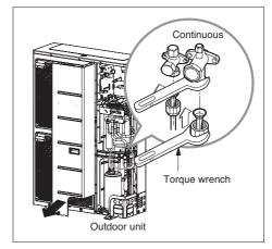
₩ When tighten the pipe, hold the haxagonal body.
