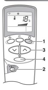
Press the START/STOP BUTTON to turn the unit on. The unit will respond with a beep.
