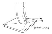
Secure the connection with a supplied screw, then insert a speaker wire from the bottom of the base.
