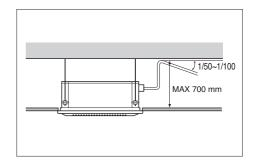
5 mm or thicker formed thermal insulator is provided for the drain pipe.
