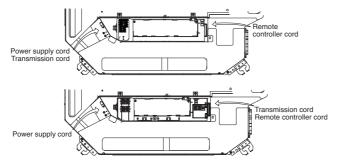
• While connecting wired remote controller, insert its connector to the "CN-REMO" housing of the main PCBA and make the remote controller cord tightly by using clamp cord.
