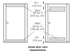
Minimum vent opening for built-in installation is 31 ½ sq. in. (200 cm<sup>2</sup>).
