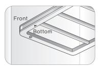
2 Insert the left shelf groove into the left shelf support, then lower the right shelf groove onto the right shelf support.
