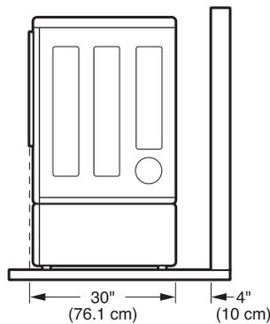
Required Dimensions for Installation With Stacking Kit
