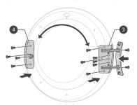
5 Remove the door catch **5** from the appliance frame by removing 2 screws and then assemble them on the opposite side.
