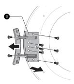
3 Remove the 3 screws from the door latch assembly 4 which is fixed between the door and the hinge assembly, and then remove the screw which is fixed on the door hook.
