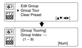
4. Use number buttons to enter the group number that is registered already then press SEL. The camera moves to the preset position in the group and the picture of the camera in that position appears on the monitor.
