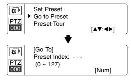
4. Use number buttons to enter the memorized preset position's index number then press SEL. The camera moves to the preset position and the picture of the camera in that position appears on the monitor.
