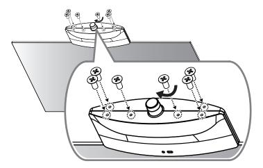
13 Prior to fastening the cover, connect the adapter and IR cable to the rotating ceiling mount board.
