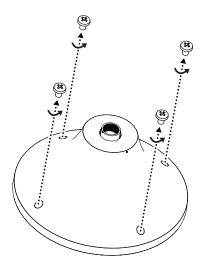
3 After connecting the pipe to the set, assemble the IR cable-linked cover and ceiling mount in order. The number of pipes connected is optional.
