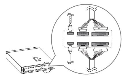
17 Attach the 16/22 pin cables using two screws (M3 x L4.5).
