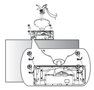
11 Cover the REAR side with the other T-con box cover and attach it using two screws (Ø3 x L10).
