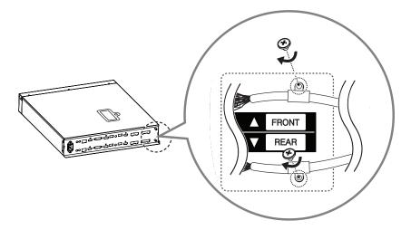
18 Position the jack cover so the cables fit into the cut spaces and attach it using two screws (M3 x L4.5).
