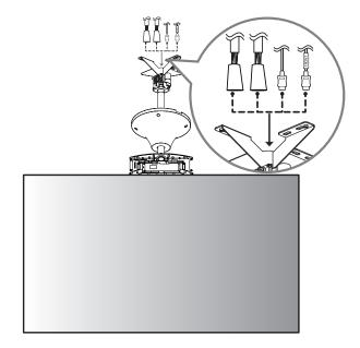
8 Connect the HDMI cable with the label marked 'FRONT' to the front side. Insert the 16/22 pin cable with the red mark into the cable holder and attach it using a screw (M3 x L4.5).
