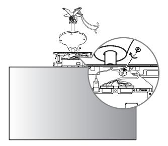
10 Cover the FRONT side with the side of the T-con box cover that has the IR receiver and attach it using four screws (Ø3 x L6) on the opposite side.
