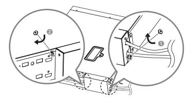
19 Attach the mounting brackets to the Signage box using four screws (M4 x L8).
