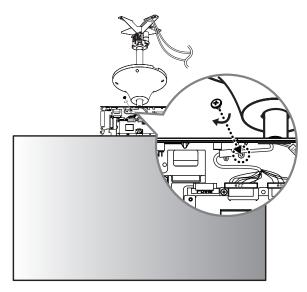
9 Connect the HDMI cable without the label marked 'FRONT' to the rear side. Insert the 16/22 pin cable without the red mark into the cable holder and attach it using a screw (M3 x L4.5).
