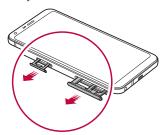
3 Put the SIM card on the card tray with the gold-coloured contacts facing downwards.
