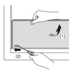
**3** Insert a small flat screw driver into the hole of the movable pin. Slide the pin to the right and remove the mini table.
