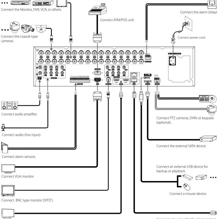
Connect network cable for client control or IP camera input.
