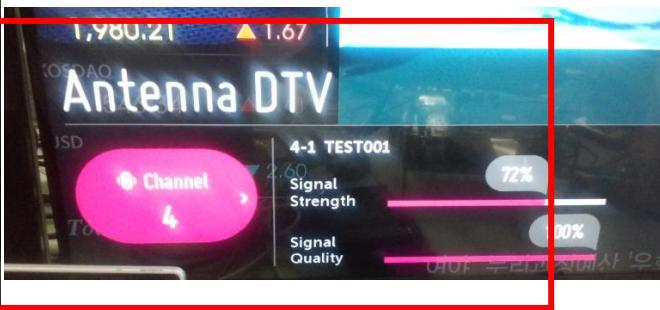
When the signal is strong, use the attenuator (-10dB, -15dB, -20dB etc.)
