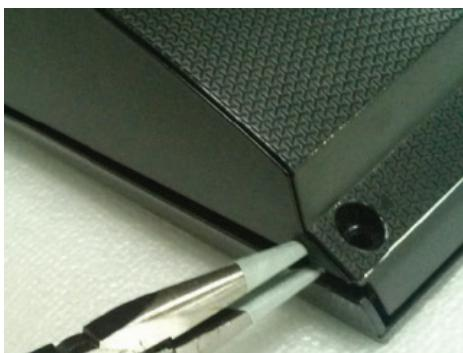
(5) Open B/C with push/pulling long nose to upper and lower sides.
