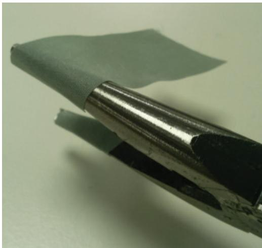
(3) Attach tape to 'Long nose pliers'
