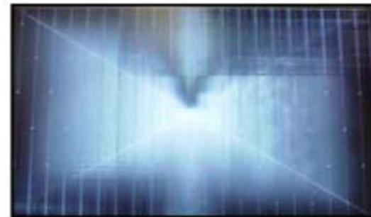
Solder defect, Short/Crack
