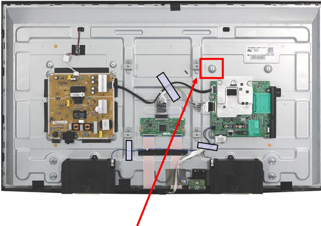
After turning on the power and disassembling the case, check with the naked eye, whether you can see light from locations.
