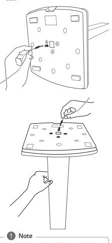
Make sure speaker cable unfolded or in straight condition before insert it to the hole.
