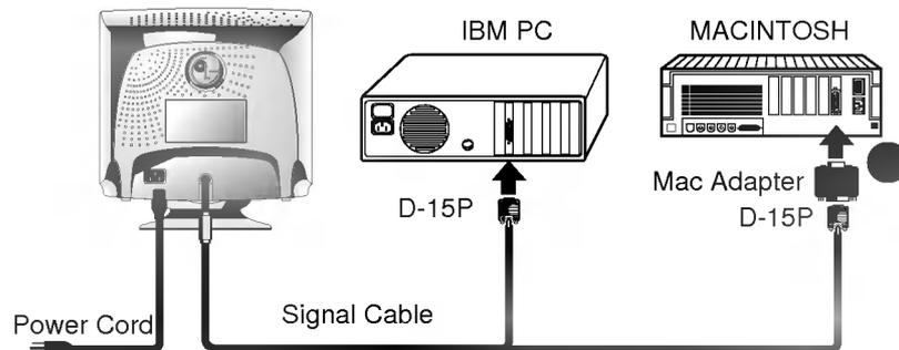
\* **NOTE** : For Apple Macintosh use, a separate plug adapter is needed to change the 15 pin high density (3 row) D-sub VGA connector on the supplied cable to a 15 pin 2 row connector.
