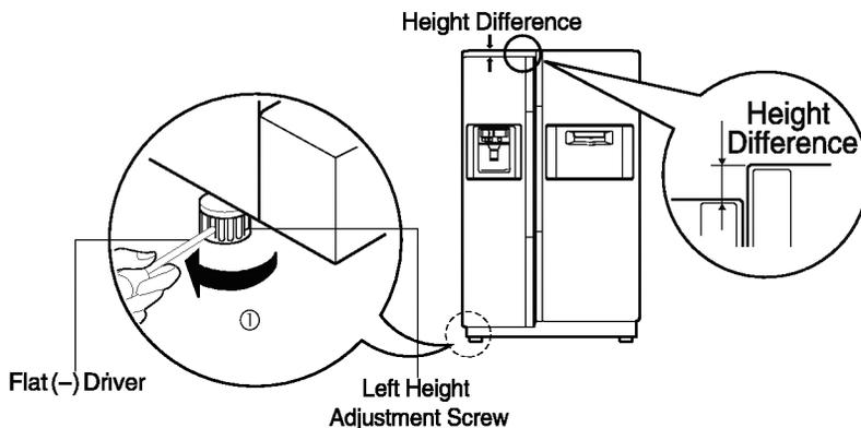
**If the freezer compartment door is higher than the refrigerator compartment door**
