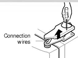
2) Remove keeper by rotating it clockwise (①) and then remove the upper hinge by lifting it up (②).
