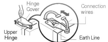
2) Remove the keeper by rotating it to counted clockwise (①) and then lifting the upper hinge up (②).
