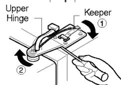
3) Remove the refrigerator compartment door by lifting it up.
