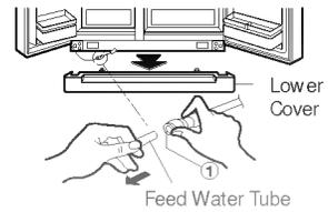
Remove the lower cover by lifting upward, and then pull up the feed water tube while pressing area ① shown in the figure to the right.
