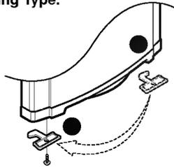
**10** Move the Cap (12) and Assemble the Freezer Door (3).
