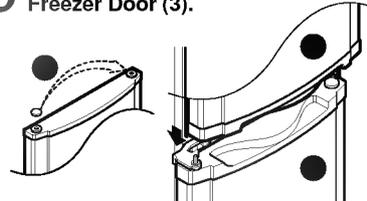
**11** Move the Pin Position (13) of the Hinge Upper.
