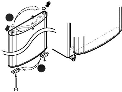
**8** Move the Cap (4) and Assemble the Hinge-C (10).
