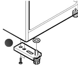
**7** Move the Cap (8), Bracket (9) of the Refrigerator Door.
