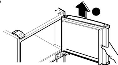
**3** Separating the Hinge-C (4) and the Refrigerator Door (5).
