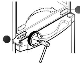
**9** Assemble the Door Stopper-F (11) for Right Opening Type.
