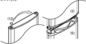
11 Move the Pin Position(13) of the Hinge Upper.
