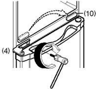
9 Assemble the Door Stopper-F(11) for Right Opening Type.
