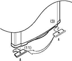
10 Move the Cap(12) and Assemble the Freezer Door(3).
