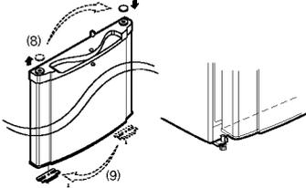
8 Move the Cap(10) and Assemble the Hinge-C(4).
