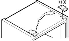
12 Assemble the Hinge Upper(2) and the Cap(1).
