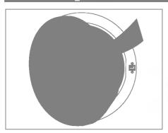
Make sure the Power switch is in the off position and always allow one to two minutes for the door safety lock to release the lock. Pull the handle to open the door.
