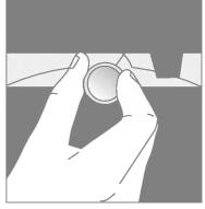
Plastic plugs, supplied inside the protective bag and designated as "P", should be placed in the safety bolt holes according to the direction shown.
