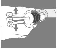
Remove transport safety bolts and rubber bushes by pulling outwards. (A up/ down action and a small squirt of washing up liquid should ease removal.)
