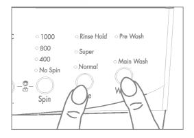
If Wash and Rinse buttons pressed same time buzzer will be off. To turn on the buzzer press again the wash and rinse buttonns at the same time.
