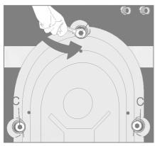
The transport safety bolts must be removed before any operation of the machine. Bolt heads, marked "C".
