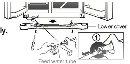
**Remove lower cover and then feed water tube**
