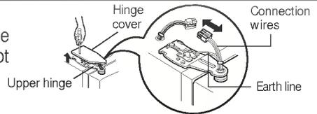
2) Remove the keeper by rotating it counter clockwise (①) and then lifting the upper hinge up (②).
