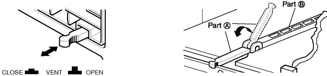
**NOTE:** Before using the ventilation feature, make a ventilaiton kit. First, pull down part ① to ② horizontal line with part ③.
