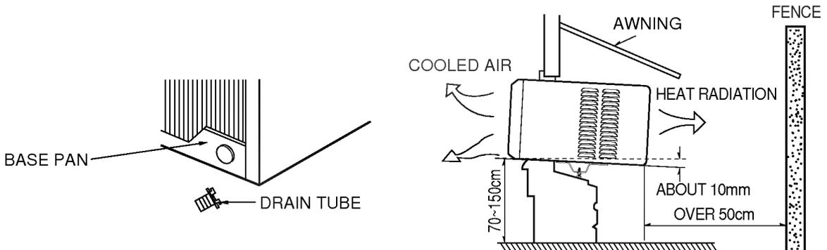
1. To avoid vibration and noise, make sure the unit is installed securely and firmly.
