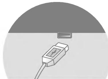
**USB downstream Ports** connect the cables from USB compliant peripherals-such as keyboard, mouse, etc
