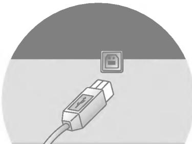
To **USB downstream port** of the USB compliant PC or another hub cable
