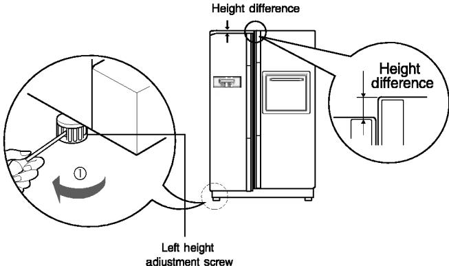
**If the freezer compartment door is higher than the refrigerator compartment door**
