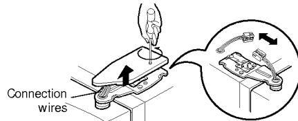
3) Remove refrigerator compartment door by lifting up.
