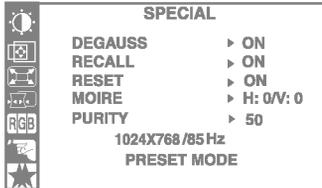
**DEGAUSS** To manually demagnetize the screen to avoid showing incorrect images or colors.
