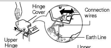
2) Remove the keeper by rotating it to counted clockwise (①) and then lifting the upper hinge up (②).
