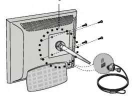
Kensington Security Slot- optional Connected to a locking cable that can be purchased separately at most computer stores
