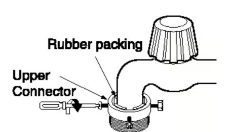
3. Push the water supply hose vertically upwards so that the rubber packing within in the hose can adhere completely to the tap and then tighten it by screwing it to the right.
