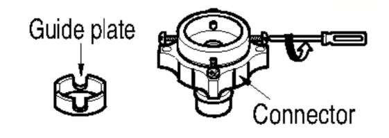
2. Push the upper connector up till the rubber packing is in tight contact with the tap. Then tighten the 4 screws.
