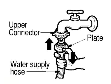
To separate the water supply hose from the middle connector shut off the tap. Then pull the inlet hose down, pushing the plate down.
