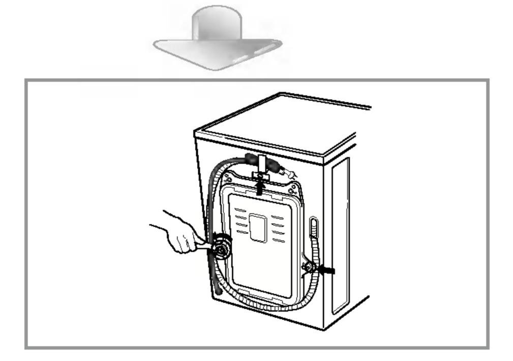
2. Unscrew the 3 bolts with the spanner supplied.
