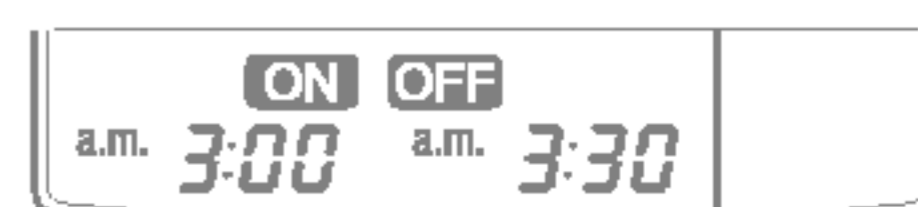
Delay ON and OFF Timer
