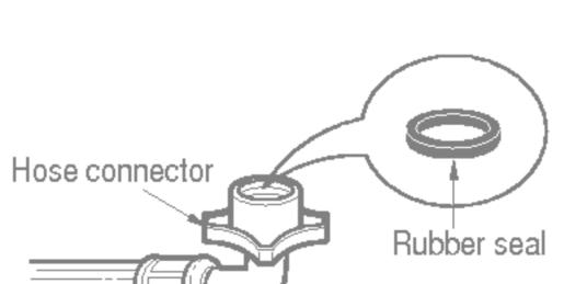
3. Connect the water supply hose to the middle connector, pushing the plate down.
