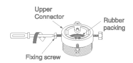
2. Push the connector up till the rubber packing is in tight contact with the tap. Then tighten the 4 screws.
