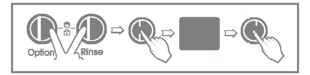
The child lock can be set at any time and it is automatically canceled when operational errors occur.
