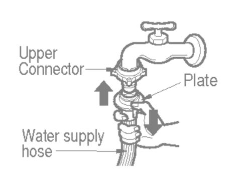
To separate the water supply hose from the middle connector shut off the tap. Then pull the inlet hose down, pushing the plate down.
