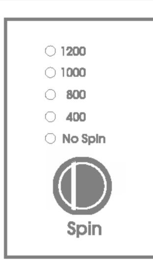
By pressing the Spin button, the spin speed can be chosen.
