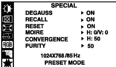
**RECALL** You can use this function to reload the modified parameters for screen display operation, as specified by the user after purchase: *Position, Size, Side Pincushion, Trapezoid* (These recalled options may differ depending on the mode selected: *Preset, User, or New*).
