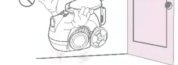
In winding the power cord, hold the plug before pressing the button of the cord reel. Do not pull the power cord beyond the red warning line; otherwise the power cord may be damaged or unable to be wound
