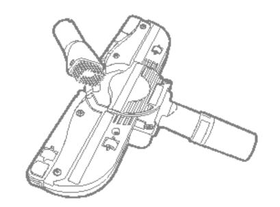
Wipe all the soiled parts of the vacuum nozzle body with a cloth.
