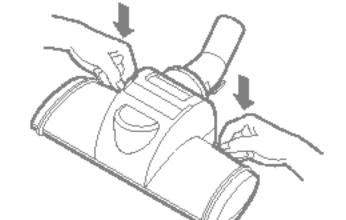
Press the button on the rear side of the vacuum nozzle to separate the bottom plate.
