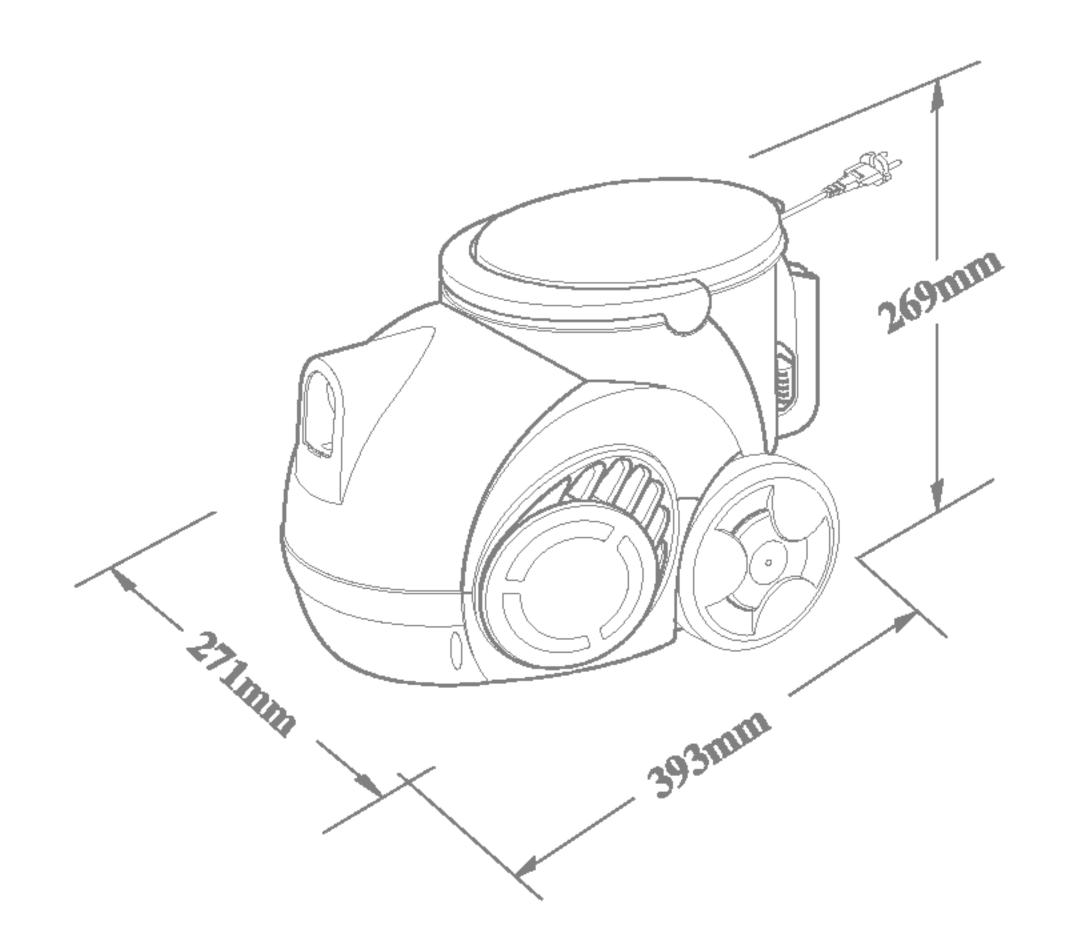
Model: V-776CAR 220V~50Hz IEC: 1500W Suction Power: 280W Net Weight: 4.5Kg Dimension: 393mmx271mmx269mm This appliance complies with the following GB Directives:
