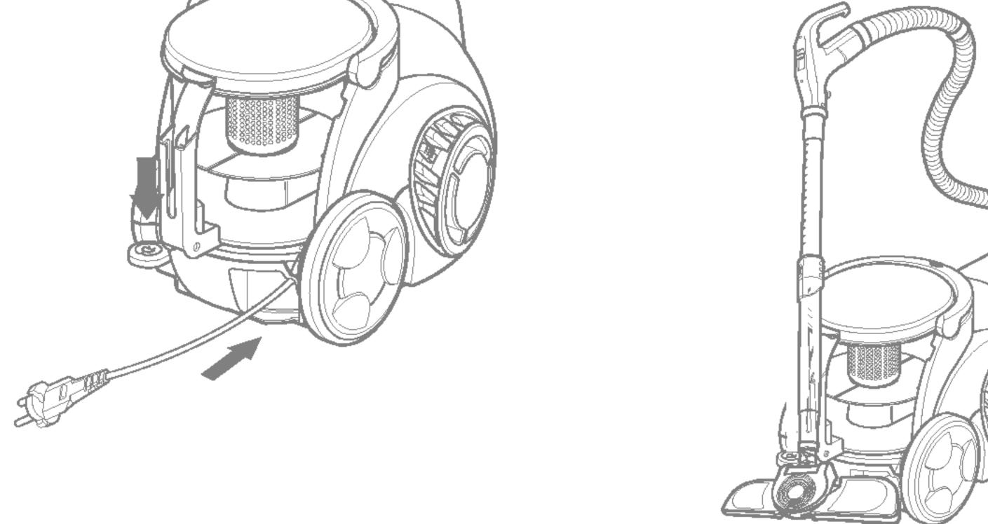
\* If the power cord cannot be completely rewound, pull out part of the cord and rewind it again.
