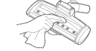
Wipe all the soiled parts of the vacuum nozzle body with a cloth. Wash the removed bottom plate with water and dry it.. Insert the attachment projections on bottom plate to the vacuum nozzle grooves.
