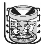
Water pours down and circulates
