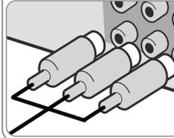
Connect the COMPONENT VIDEO (PROGRESSIVE SCAN) OUTPUT jacks on the unit to the corresponding input jacks on your TV using a Y PB PR cable.
