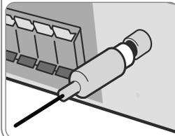
FM - Connect the FM aerial. The reception will be its best when the two loose ends of the aerial are in a straight and horizontal line.
