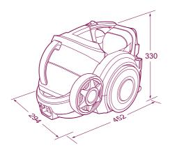
Model: V-KC902HE 220V~ 50Hz IEC: 1800W MAX: 2000W Suction Power: 300W Net Weight: 6.5 Kg Dimension: 294mm x 452mm x 330mm This appliance complies with the following GB Directives: GB4706.1-2005 GB4706.7-2004 GB17625.1-2003 GB4343-2003
