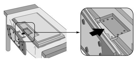
**3.** Use the screws to secure the stand on the rear side of the product as shown in the diagram.
