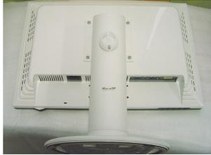
2. Separate the stand using a screwdriver as shown in the picture.
