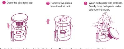
Avoid picking up hard, sharp objects with the cleaner. They may damage the cleaner and the tank.
