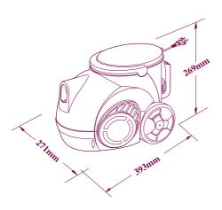
Model: V-774CAY 220V~50Hz IEC: 1200W MAX: 1400W Suction Power: 300W Net Weight: 4.5KG Dust Capacity: 1L Dimension: 393mmx271mmx269mm This appliance complies with the following GB Directives: GB4706.1-2005 GB4706.7-2004 GB17625.1-2003 GB4343-2003
