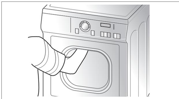
4. Remove the current bulb turning it to Counter clockwise direction.
