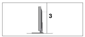
Use a sturdy rope to tie the product for alignment. It is safer to tie the rope so it becomes horizontal between the wall and the product.
