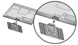
Fix the 4 bolts securely using the holes in the back of the TV.
