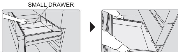
3. Install the white plastic drawer in reverse order, then install the small drawer. Pay attention to the direction when installing the small drawer.
