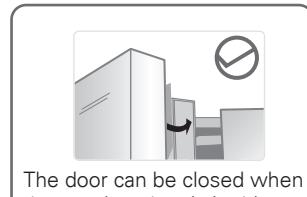
The door can be closed when the rotating plate is in this position.
