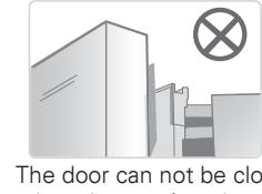
The door can not be closed when the rotating plate is in this position.
