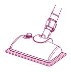
▶ The steam brush head shall be maintained on the specific pad rather than directly on the floor when it is still hot; otherwise it may damage the floor.
