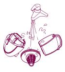
Cleanse the dust box, separator and its cover with running water.
