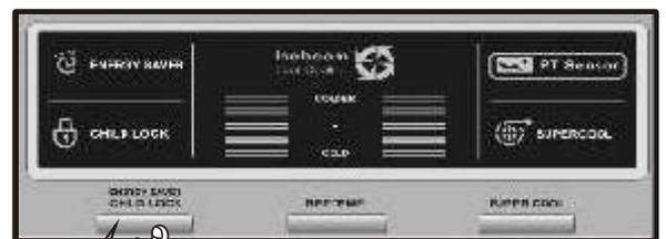
Press this button for 5 seconds and The CHILD LOCK lamp will turn ON. Press the button for 5 seconds again and the CHILD LOCK lamp will turn OFF.
