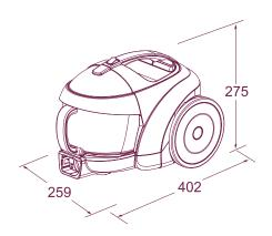
Model: VC3016NND 220V~ 50Hz IEC: 1400W MAX: 1600W Suction Power: 300W
