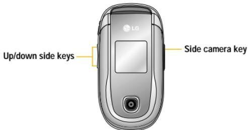
1. Press the side camera key to activate the display on the front screen.
