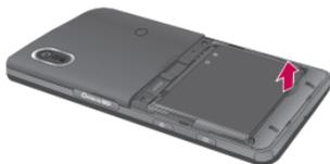
**⚠ WARNING:** Do not remove the battery when the phone is switched on, as this may damage the phone.
