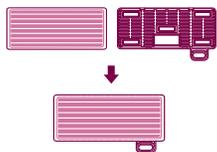
2. After the mop nozzle matches with the mop board, connect the mop nozzle from the top down. When you hear a sound of Ta Ta, it means the connection is ok.
