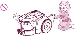
Do not pull or carry by cord, use cord as a handle, close door on cord or pull cord around sharp edges or corners. Do not run appliance over cord. Keep cord away from heated surfaces.
