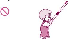
Do not operate the appliance for long when the nozzle inlet or nozzle outlet is blocked, which may have it deformed or damaged.
