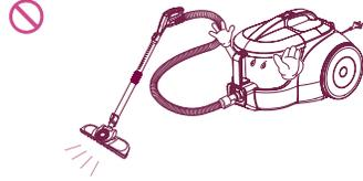
In using the appliance, pay attention to the electrostatic effect generated on the telescopic tube and cleaner body.
