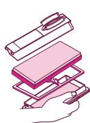
1 Put the filter into the case.
