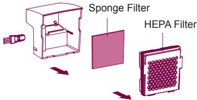
After separating the filter from dust bin, separate sponge filter from HEPA Filter as in the figure.
