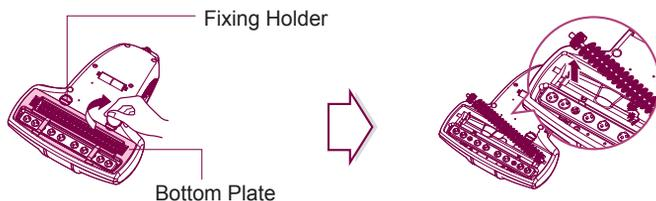
Place a soft cloth on the floor, and flip over the main body on it. Check for foreign objects, turn the 2 fixing holders 90° clockwise with linear shape screwdriver or similar tools and separate the bottom plate by pulling it up. Hold the roller brush and separate it by lifting it up.
