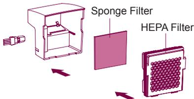
Assemble in the reverse order of disassembly.
